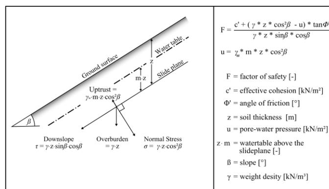
Figure 11: Principle for the calculation of the factor of safety  $F$  for every raster cell (Selby 1993)
