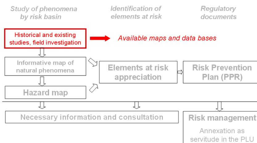
Figure 49: The first step of hazard mapping
