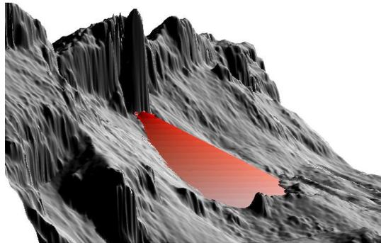
Figure 10: The viewshed function identifies all raster locations to be seen from appointed starting points with defined global angle.
