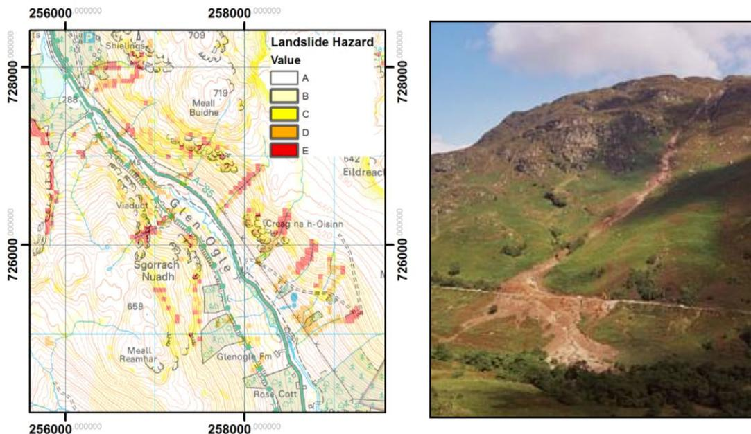
Figure 45: Extract from the Debris Flow Susceptibility Layer along with b) the Glen Ogle debris flow of 2004
