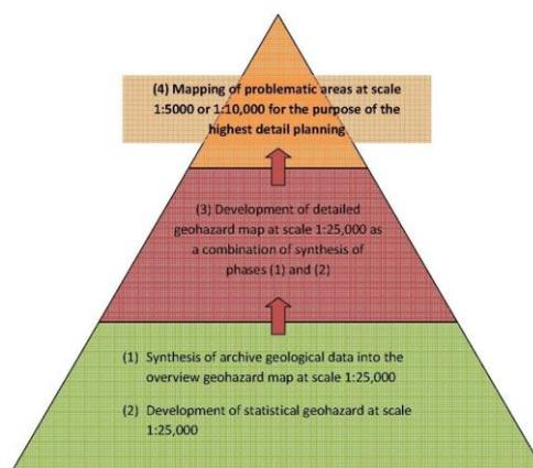
Figure 41: Schematic diagram of the process of production of landslide and rock-fall susceptibility at the municipal scale (1:25.000) (Bavec et al., 2005).
