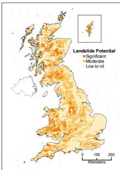
Figure 43: GeoSure layer showing the potential for landslide hazard.
