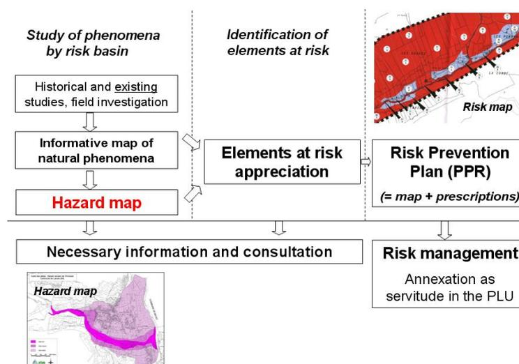
Figure 48: Positioning of the hazard map within the general procedure of PPR elaboration
