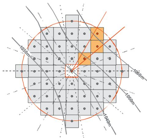
Figure 12: Calculation of accumulation: for the central cell with exposition of 210° –230° the 20° sector identifies 3 cells that are either starting zones or already show accumulation (orange cells)
