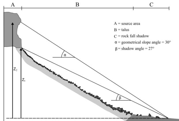
Figure 9: Global angle models: shadow angle ( $\beta$ ) and geometrical slope angle ( $\alpha$ ) (Meißl 1998, modified)
